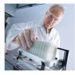
**OPUS®RoboColumn®** is a miniaturized column on a 96well plate used with robotic fluid handlers for automated, parallel chromatography resin screening and sample preparation.
