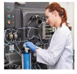
**OPUS® 5** has an internal diameter of 5 cm, ideal for process development assessment of chromatography scale-up prior to clinical or commercial manufacturing.
